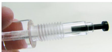
Fig. 2— Installing the Side Fitting Plug.
