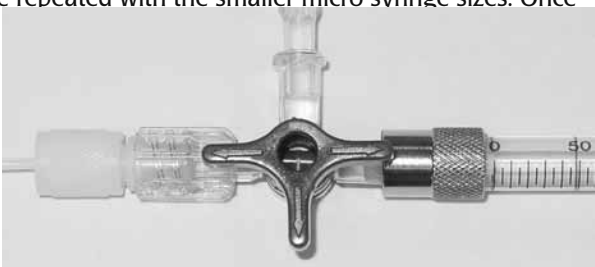
Fig. 6—Male and female luers are open (MF position)
