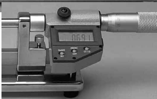
Fig. 2— On the DMP the micrometer has a digital display
