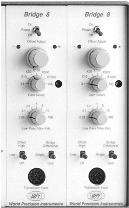
Fig. 1—Up to eight rackmountable ISO-DAM8A and Bridge8 modules can be combined in a single chassis.
