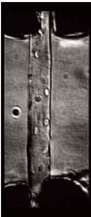
Above—A single FDB skeletal muscle cell is held by two microtweezers in the Cell Tester unit.
