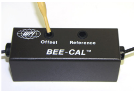
Fig. 4—Use a potentiometer adjustment tool to turn the Offset control screw until the pH meter displays 7.0pH.
