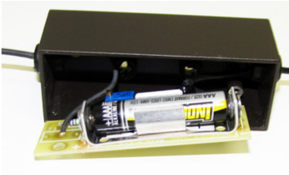
Fig. 7—The battery is located under the circuit board.
