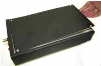
Fig. 6—If you tip the box upside down, the back end of the lid opens and you can slide it off the box.
