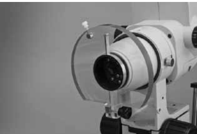
Fig. 9– Tool holder plate installed
