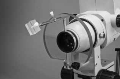
Fig. 10– Tool holder bar installed
