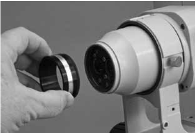
Fig. 7– Installing the ring light adapter
