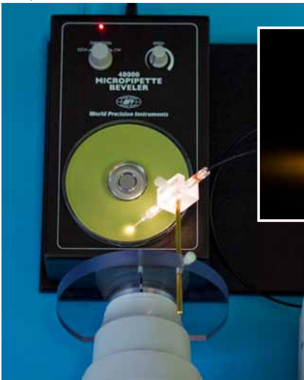
Fig. 12 – (Left) 48000 Beveler in use as seen from above
