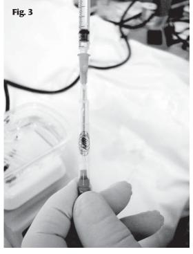
that no air is trapped in the cartridge. Now, screw the electrode into the cartridge until it is snug or will go no farther (Fig. 4). To remove the needle, make sure that the syringe is firmly on the cartridge and slowly inject more gel as you move the needle out of the cartridge. Holding the cartridge vertically, check to see that there are no air bubbles in
