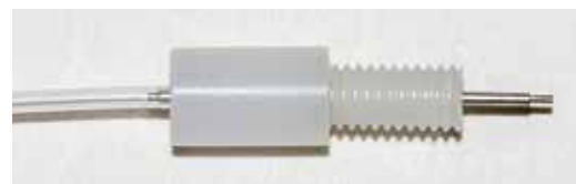
Internal cannula secured with fixing screw.
