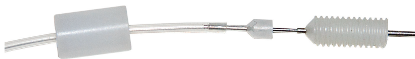
Cannula assembly: fixing screw, internal cannula with attached tubing, and guide cannula.
